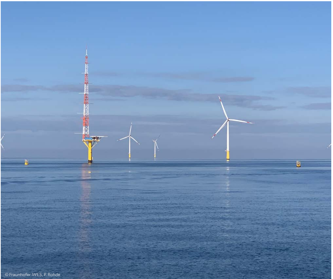
Two Fraunhofer IWES wind lidar buoys during performance verification next to the FINO3 offshore met. mast in the German Bight
