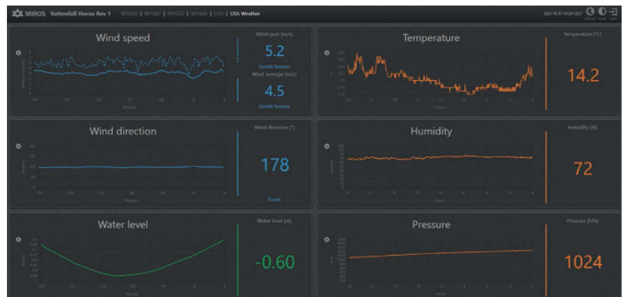
With the help of IoT-enabled Miros RangeFinder sensors distributed across the wind farm, the various Vattenfall project teams can simultaneously view the actual sea state conditions across the entire site on real-time dashboards, accessible anytime on any device. Live data from this project can be seen at miros.app
