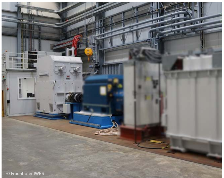
The HiL-GridCoP test bench for performing grid compliance tests on subsystem level of high-speed generator-converter systems
