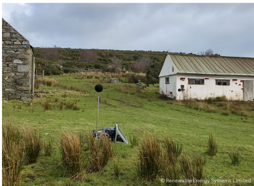
Typical acoustic monitoring device installed on-site
