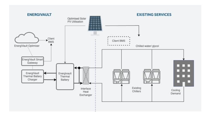
It stores latent heat in freezing tiny water particles and this characteristic allows high-efficiency charging of the thermal battery, compared to equivalent solid ice storage systems, and ultra-high discharge cooling for peak and transient cooling demand management.
