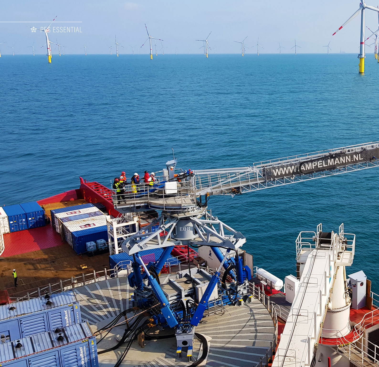
Capable of withstanding some of the roughest sea conditions, the E1000 can transfer personnel as well as cargo up to 1 ton
