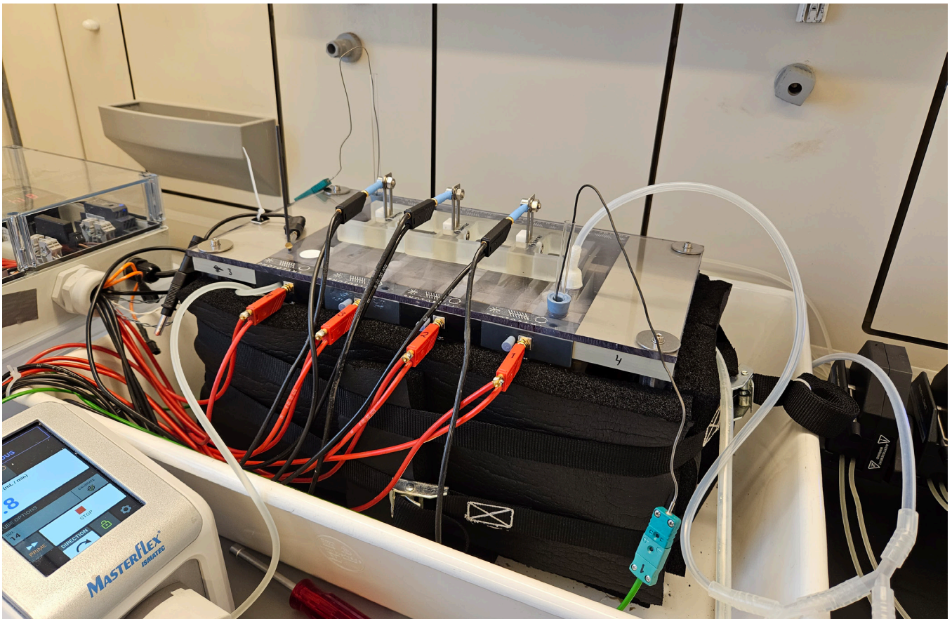
Image 7: Test equipment at Sintef for electrowinning of silver
