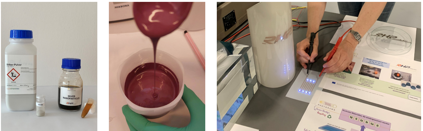
Image 8: Transformation of recycled silver into high value products, such as conductive pastes, silver nanoparticles and nanowires
