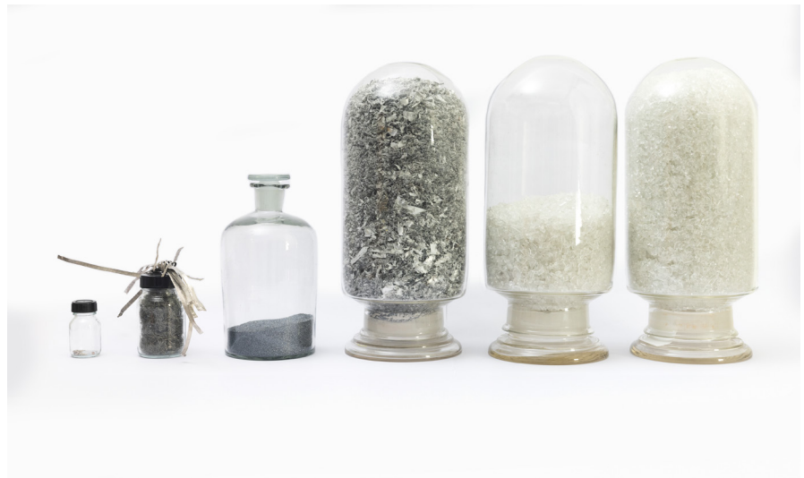
Image 2: From left: 6 g silver, 0.05 kg copper, 0.5 kg silicon, 2kg foils, 14.5 kg glass
