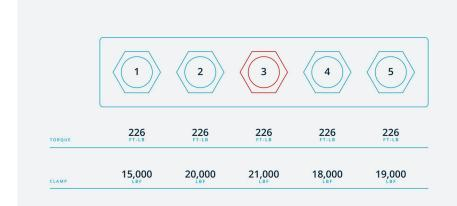
These variables, such as lubrication, diameter and thread pitch variance, atmospheric conditions, contaminants, tool calibration, and even thread wear, can result in clamp scatter of 30% or more. Clamp scatter of this magnitude is a challenge for joint designers because it can mean that the joint is not fastened as tightly as it could be.
