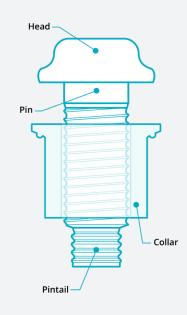
loading is put on the bolt, which will subject it to fatigue.
