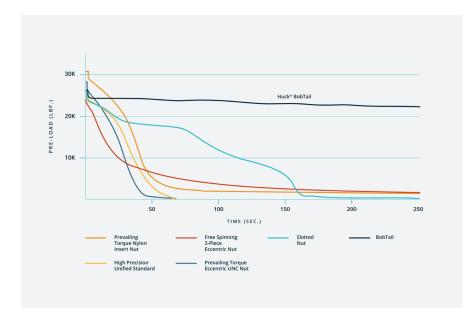
a gap between the crest of the bolt thread and the nut. When the vibration force acts perpendicular to the bolt, the nut can shift side to side and eventually 'back off'.
