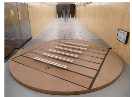
Wind tunnel testing of scale tracker models to determine aeroelastic performance
