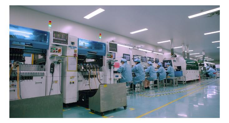
These procedures ensure that every micro-inverter product undergoes stringent quality inspection processes, including Automated Optical Inspection (AOI), Functional Testing (FCT), Aging Testing. Additionally, advanced management methodologies such as 'Kanban Management', '5S Principles' and 'Six Sigma Principles' are employed to further enhance product quality and reliability.
