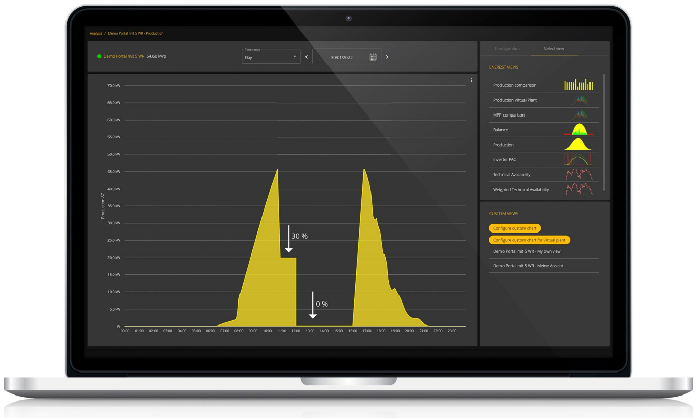
Figure 1: Feed-in management means the controllability of decentralised generation plants. There can be different levels of control, as can be seen in the picture, e.g. a reduction to 30% or even 0%.
