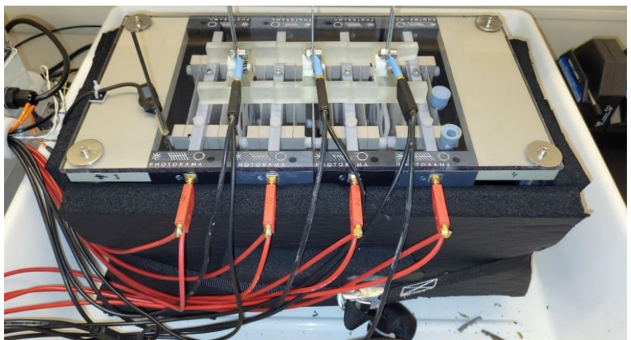
Electrowinning cell for Ag production at SINTEF
