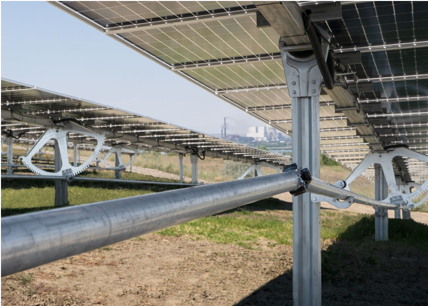
The decoupled drive design and universal joints allow L:TEC to follow slope changes up to 36% after every string
