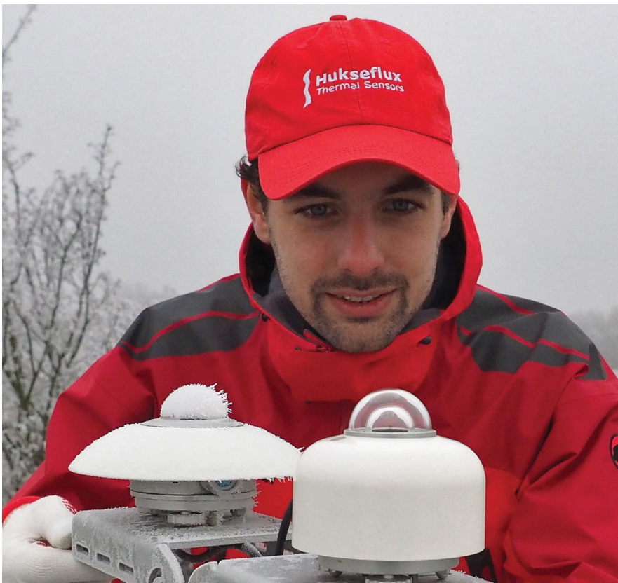
Hukseflux pyranometers are heated. Heating counters frost and dew deposition. The image shows a clear difference between a non-heated pyranometer at the back and a heated Hukseflux pyranometer at the front
