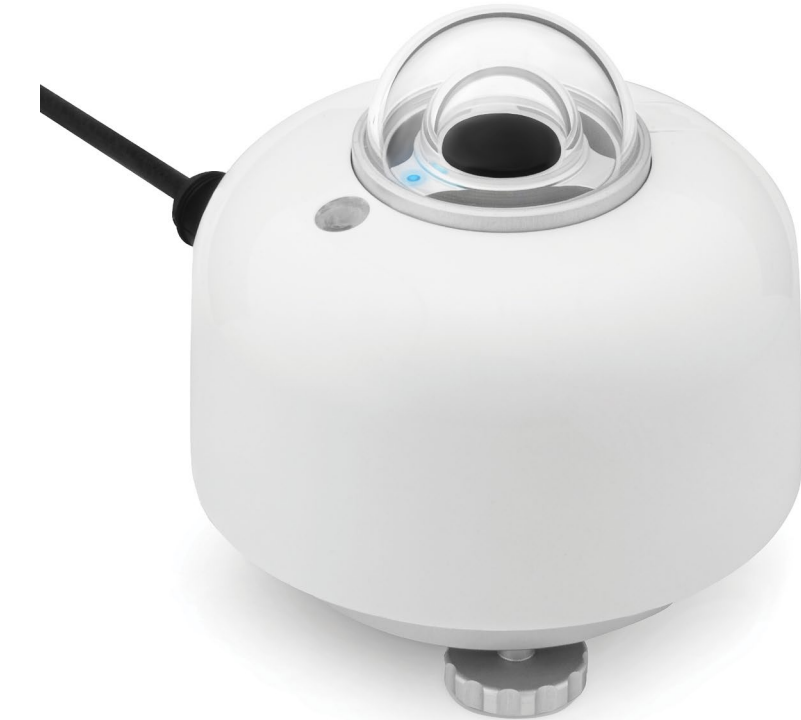
New from Hukseflux: the SR300 industrial pyranometer with heating, tilt sensor and status LED. With integrated surge protection, this is designed to withstand the extreme conditions encountered on PV power plants
