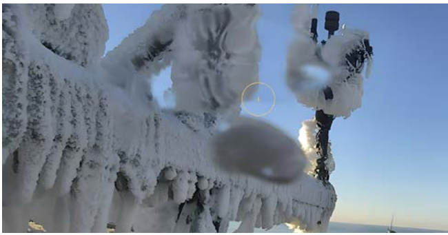
A nacelle surface without NEINICE coating covered in a thick layer of ice. These photos were taken on the same day.
