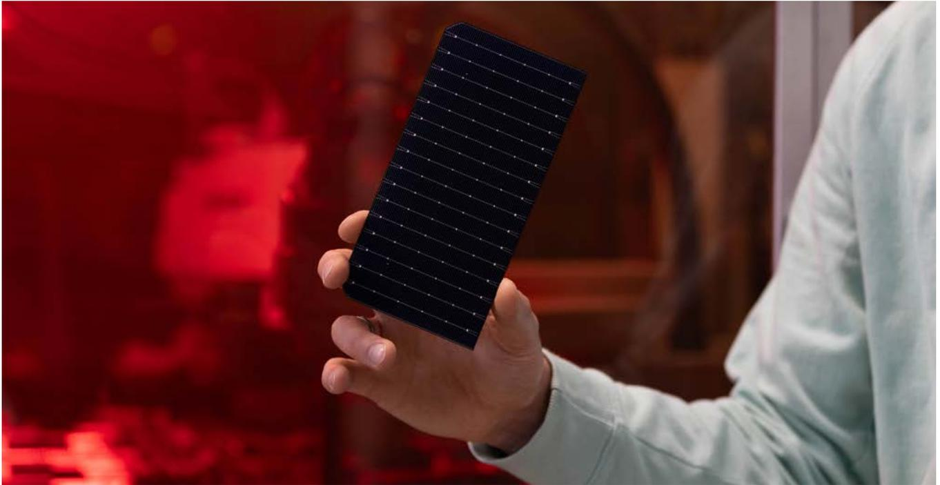
promise higher efficiencies and are less susceptible to power losses. TopCon is rapidly gaining market share and in comparison, to PERC or HJT (Heterojunction) cell technology has emerged as the frontrunner to be the dominant cell technology in the evolution of photovoltaics.
