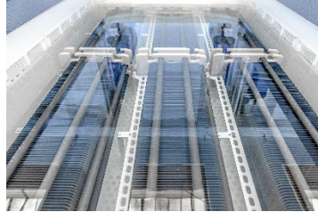
BatchTex N600 – Large volume solar cell manufacturing tool
