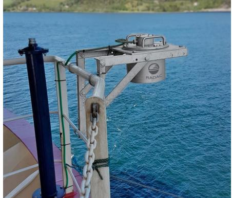
field experiment. This involved a comparison between data gathered from a Directional Waverider buoy and data obtained from the WaveGuide. This comparative study took place at Prinses Amaliawindpark, situated 25 kilometres off the Dutch coast. Over the course of several months, two variations of the Directional WaveGuide were evaluated alongside a Directional Waverider.
