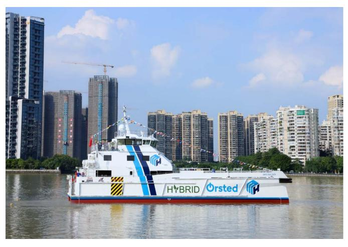
For the two new builds the power of plenty system is already a built-in feature. 'We have four separate powertrains, supplied with power from nine individual power
