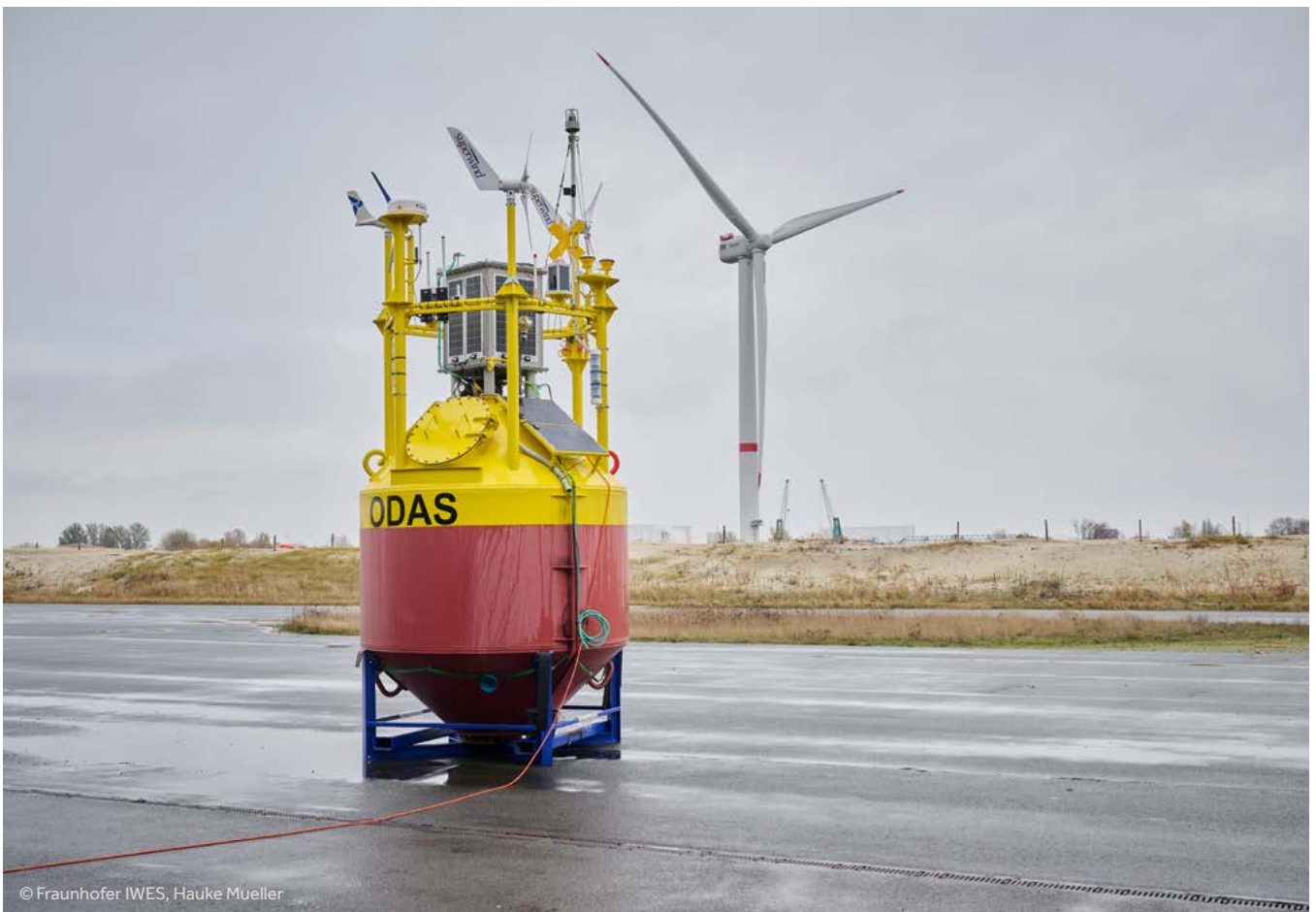
Fraunhofer IWES wind lidar buoy during final factory acceptance
