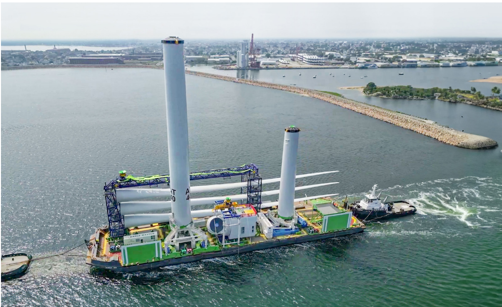
Photo: the BM-Feeder with tower seafastening and tower section.
