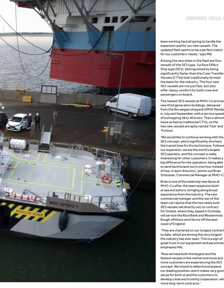
The newest SES vessels at MHO-Co are two new third generation buildings, delivered from the Norwegian shipyard UMOE Mandal in July and September, with a service speed of a whopping 38 to 40 knots. That is almost twice as fast as traditional CTVs, so the two new vessels are aptly named 'Fast' and 'Furious'.
