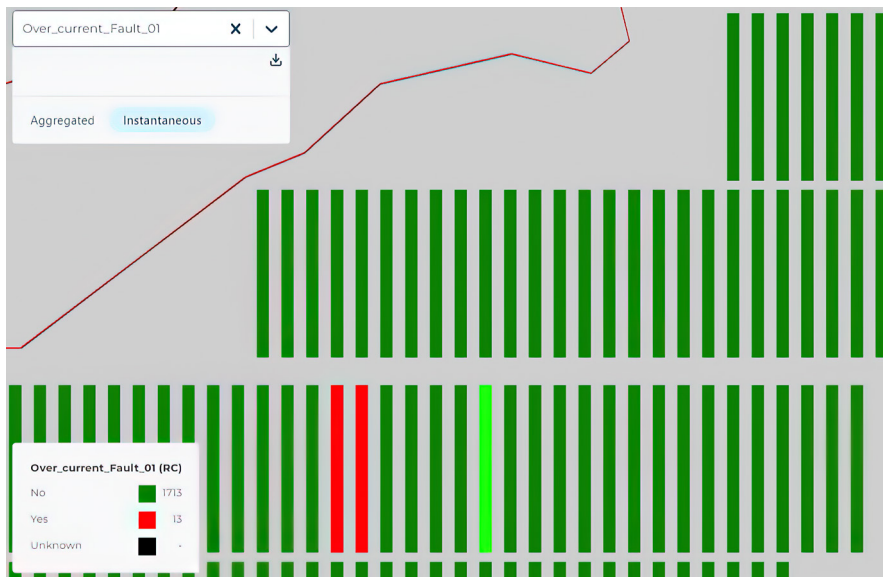
Figure 3: SUNOPS Model Viewer shows all trackers and arrays, enabling field teams to easily locate the trackers in need of repair
