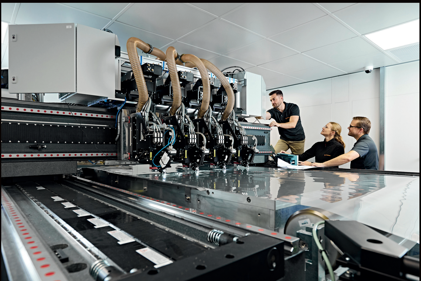
The microFLEX PV processing area: up to 12 laser heads processing substrates up to 1,400 mm in step-and-repeat-mode
