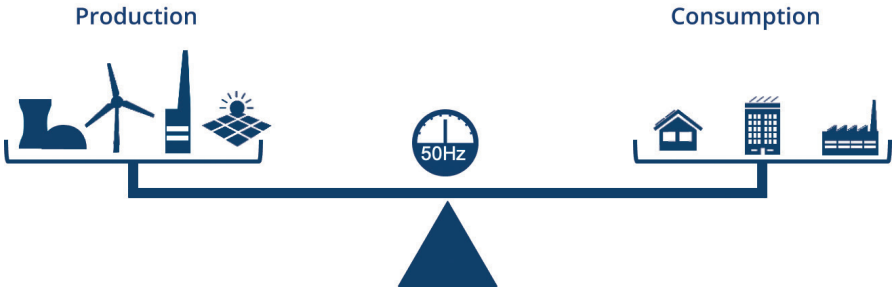
How the grid operators ensure the balance of the power grid, for voltage and frequency. The aim is to keep supply, that is the production of electricity and demand, or the consumption of electricity, in balance
