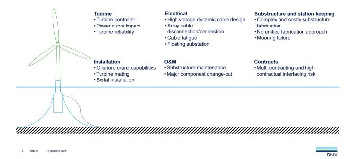
conditions. New technical, supply chain, and logistical issues will arise as floating wind evolves toward larger wind farms (800+ MW) with bigger turbines (15+ MW).
