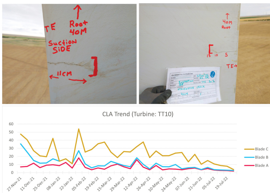
Figure 6: CLA historical trend of Turbine TT10 since system installation. The CLA trend shows increased activity of blade C, where a Trailing Edge (TE) crack in pressure and suction sides (around 32m from the root) was observed after inspection
