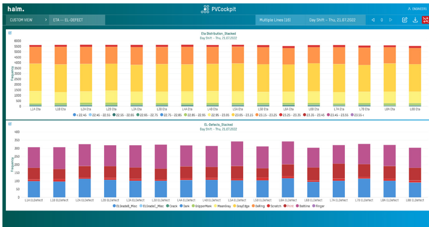
Figure 1: The top diagram shows the assigned EL quality classes of 16 lines. The lower diagram shows in detail which defects occurred in all B-quality cells
