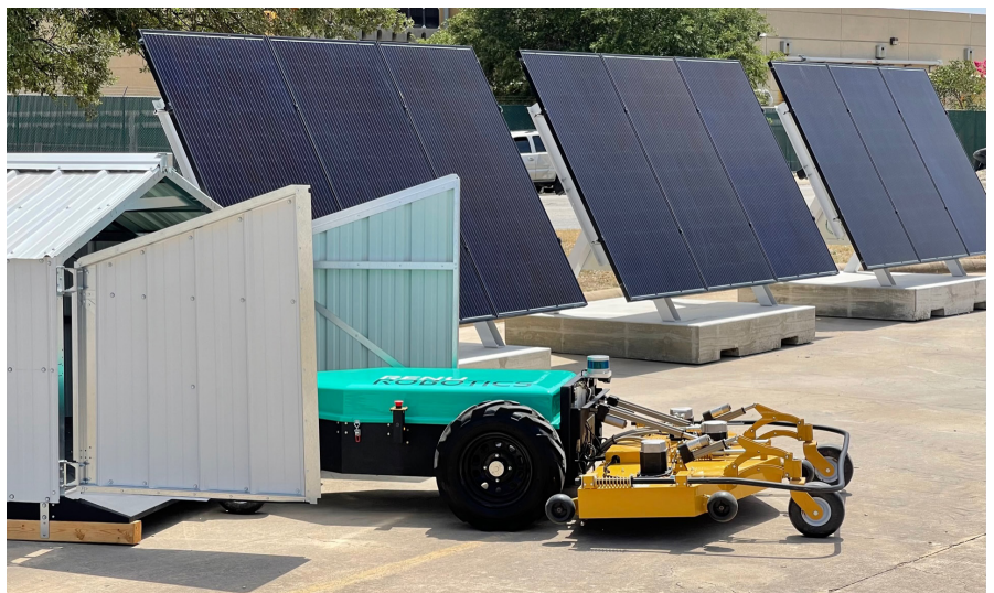
Renu Robotics' ecosystem complete with Recharge Pod, Renubot and Solar Charger, consisting of three solar skids
