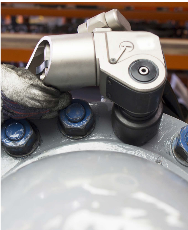
A typical scenario where fingers can be trapped and damaged as the user moves the tool
