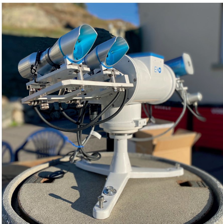
STR-22G Sun Tracker & MS-57 Pyrliometers at IPC 2021 in Davos, Switzerland
