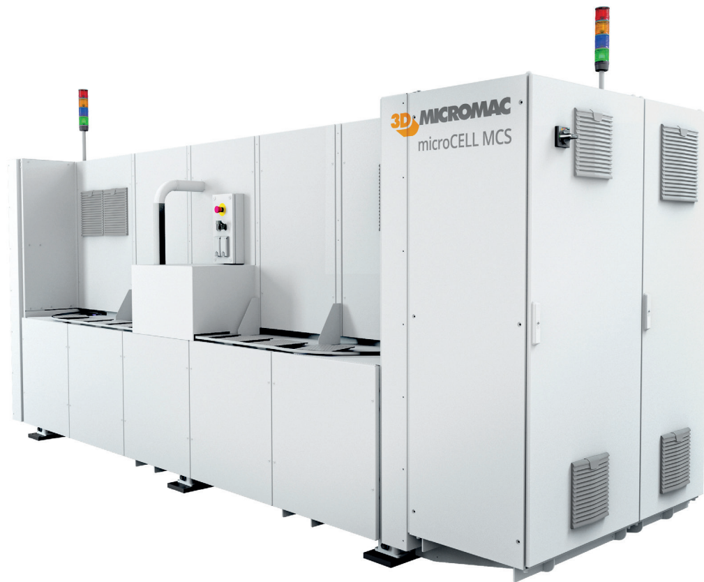
Fig 4: The new microcell MCS laser cutting system by 3D-Micromac. The new tool enables highest throughputs of more than 6,000 wafers per hour by using TLS
