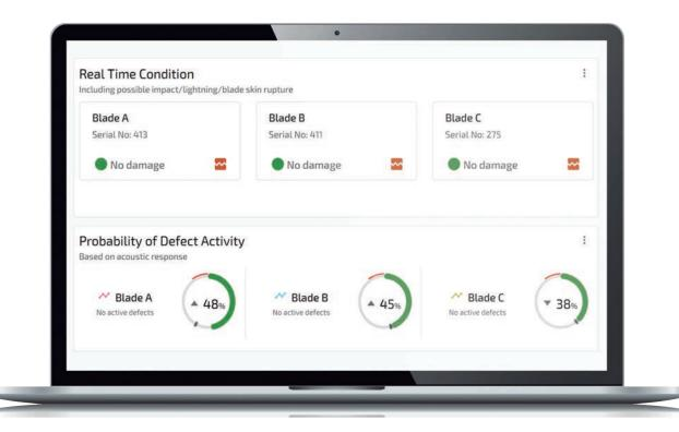
The Sensoria Insights data portal enables operators to prioritize blades for inspection by visualizing blade integrity data and alerting personnel to potential concerns
