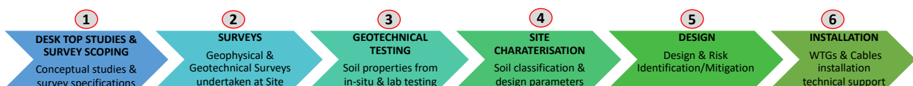
Figure 1. Key stages in an offshore windfarm project where geotechnical consultant's input is critical
