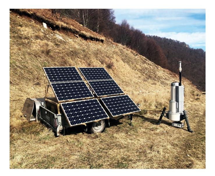
across the full swept area of a turbine rotor and beyond, even for the much larger wind turbines anticipated in future. Able to define wind characteristics well above the height of a conventional met mast, lidar capabilities fit well with the broad trends for ever bigger wind turbines.
