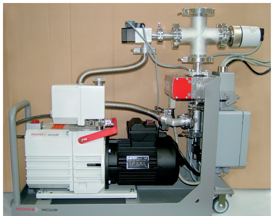
Fig. 1 Customized pumping cart for solar receiver degassing
