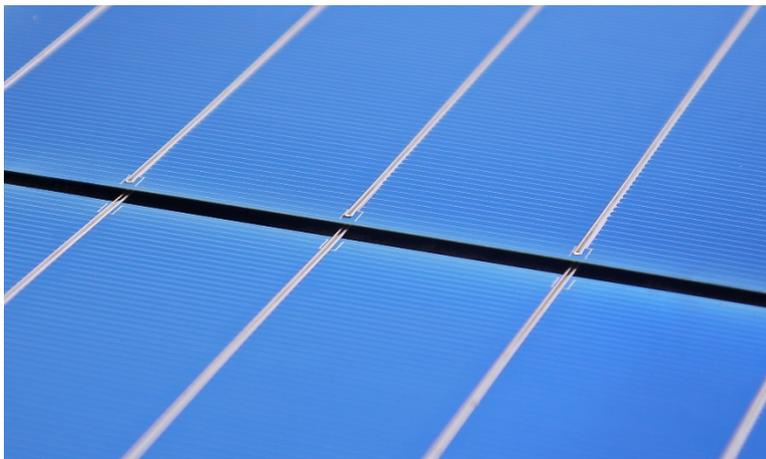
Interconnected solar cells manufactured at Fraunhofer ISE's Module-TEC. PV modules manufactured in Europe have a 40 percent smaller CO<sub>2</sub> footprint than their Chinese counterparts. © Fraunhofer ISE
