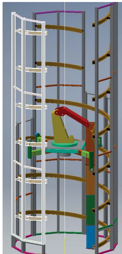
Self-positioning crane to rail. White: shell sizing
