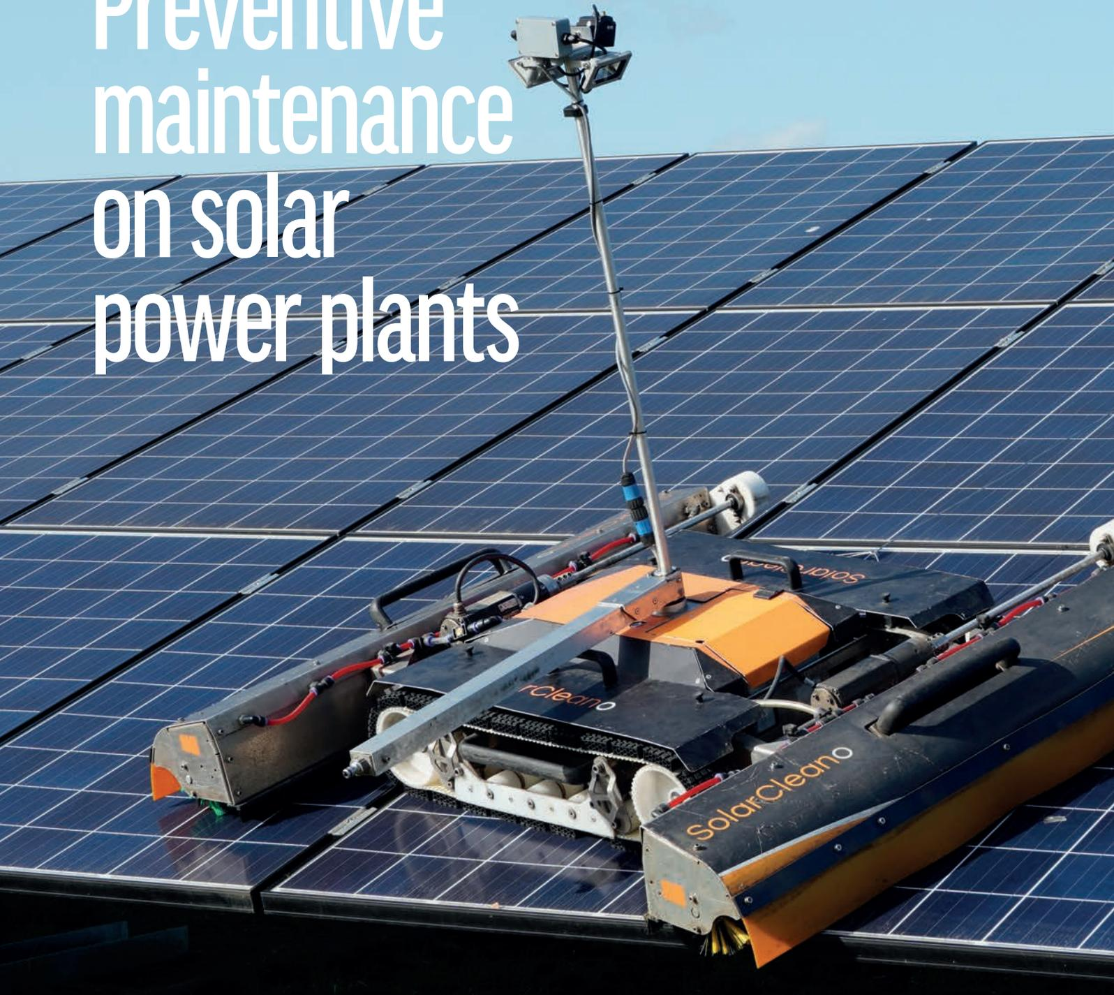
There are 4 common types of maintenance: corrective maintenance, preventive maintenance, risk-based maintenance and condition-based maintenance. The solar panel cleaning robot from SolarCleano is one of the key elements of predictive maintenance for solar power plants.
