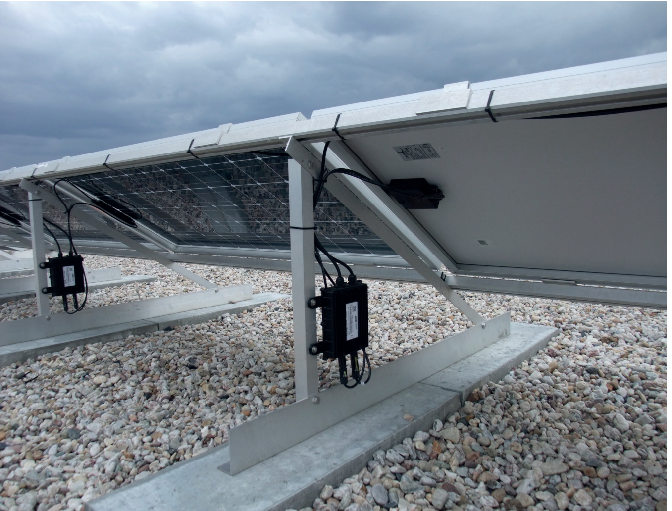
SolAround bifacial/monofacial comparative test installation - Adlershof, Germany
