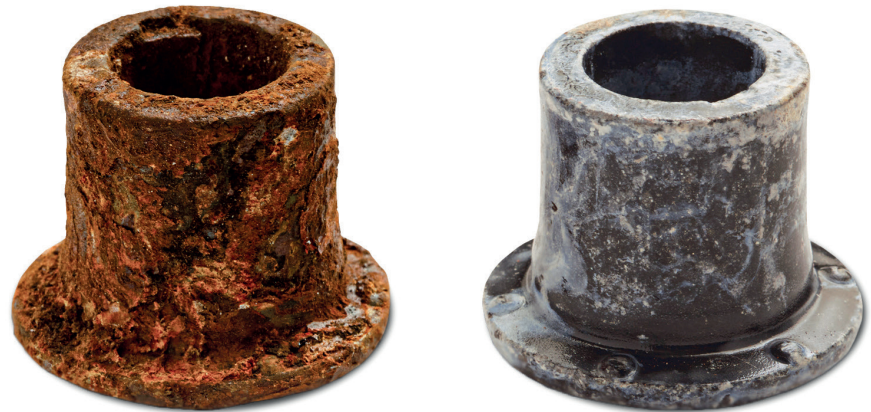
Figure 5: With and without 1000 Hour Corrosion Protection
