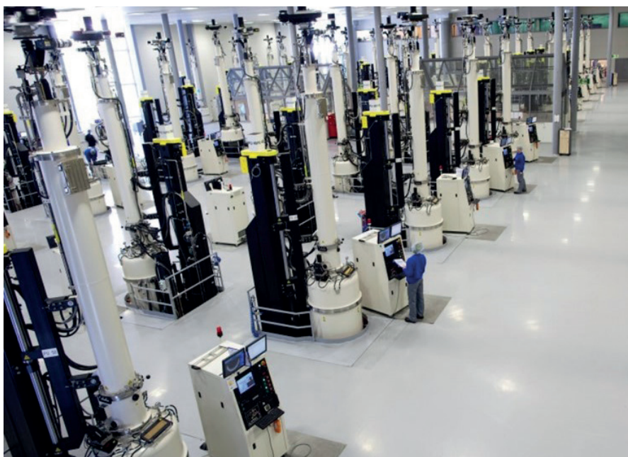
CZ furnace hall
