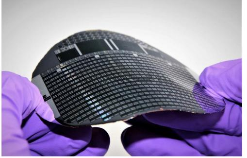
The Fraunhofer ISE research team achieved a record conversion efficiency of 68.9% under monochromatic laser light with a new thin film photovoltaic cell based on gallium arsenide. ©Fraunhofer ISE / Henning Helmers
