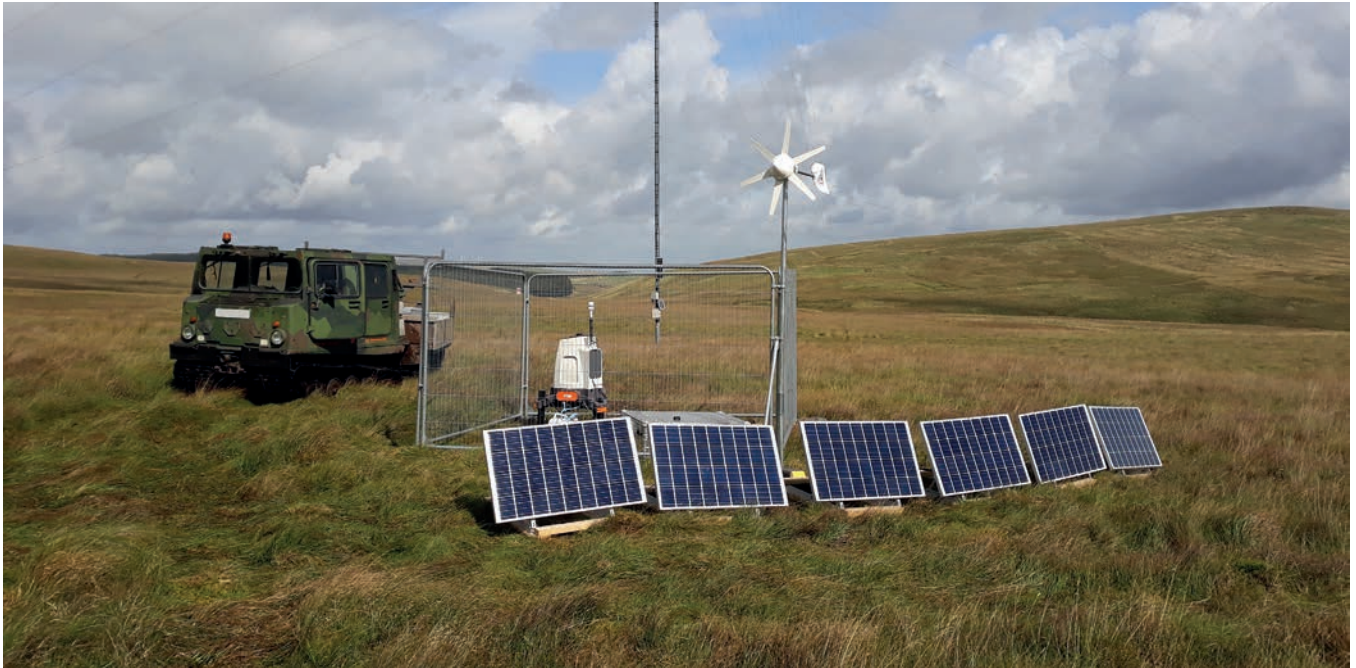
ZX 300 validating shear profile of met mast and above up to 200m+
