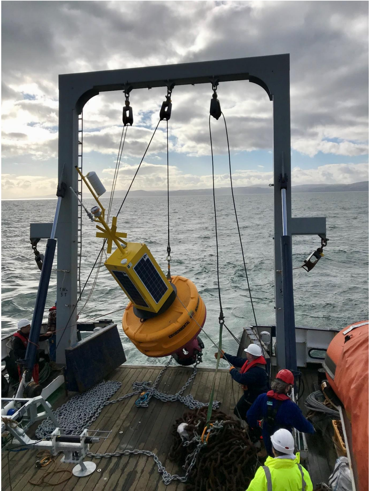
Deployment of Coastal Observatory data buoy at Constable Bank, North Wales CoastalObservatory Monitoring buoy deployment, Constable Bank
