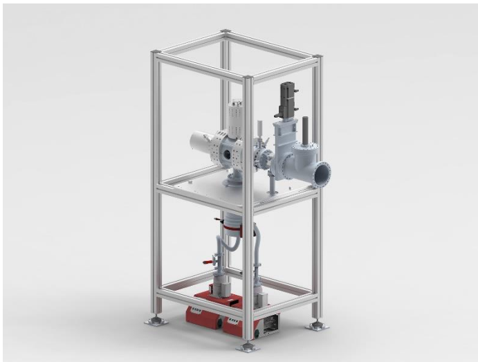
Caption: DREEBIT ion beam system for generating charged particles for the experiment
