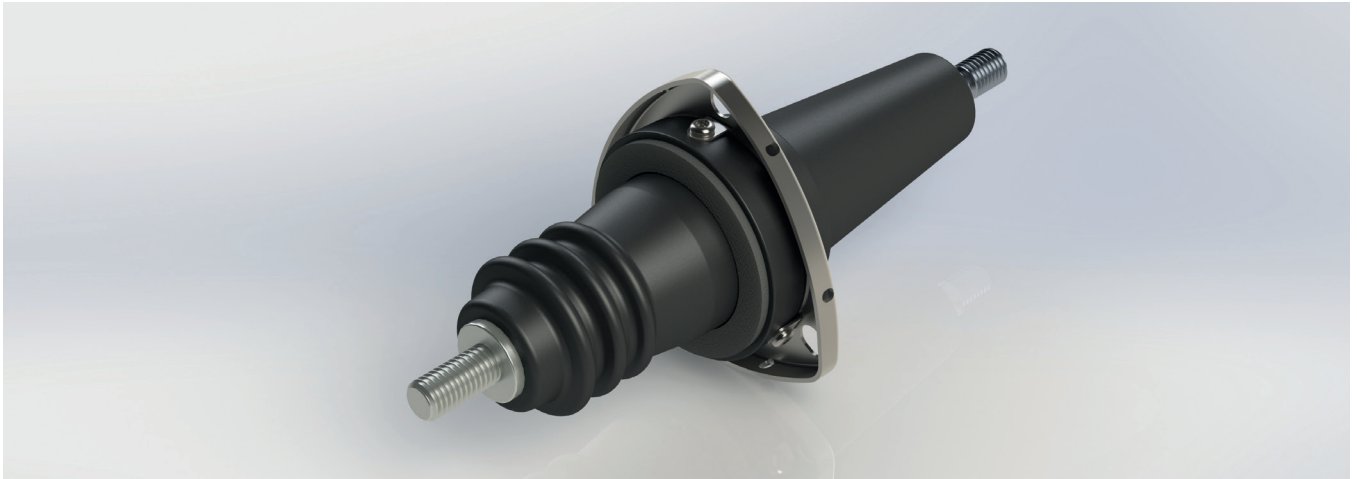
38KV 200KV BIL 600A plugin epoxy bushing 155C rated operating temperature
