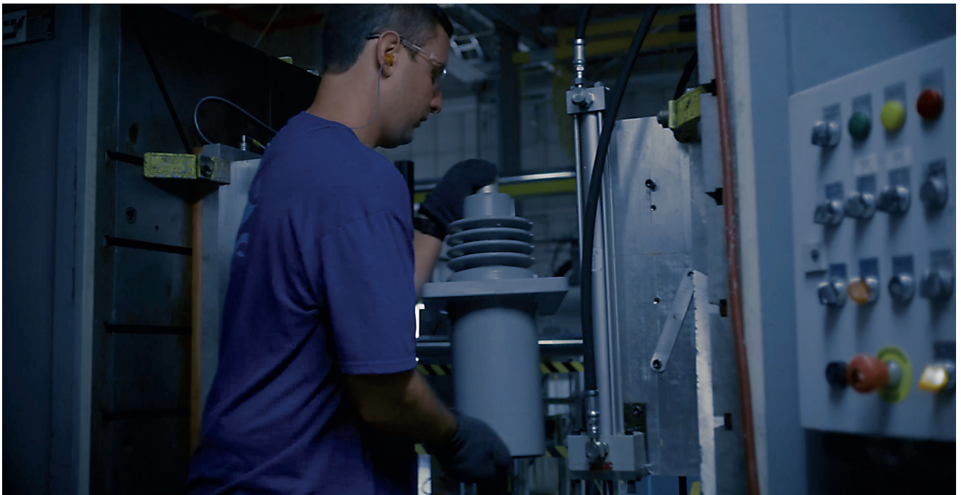
Epoxy resin customized mold press
