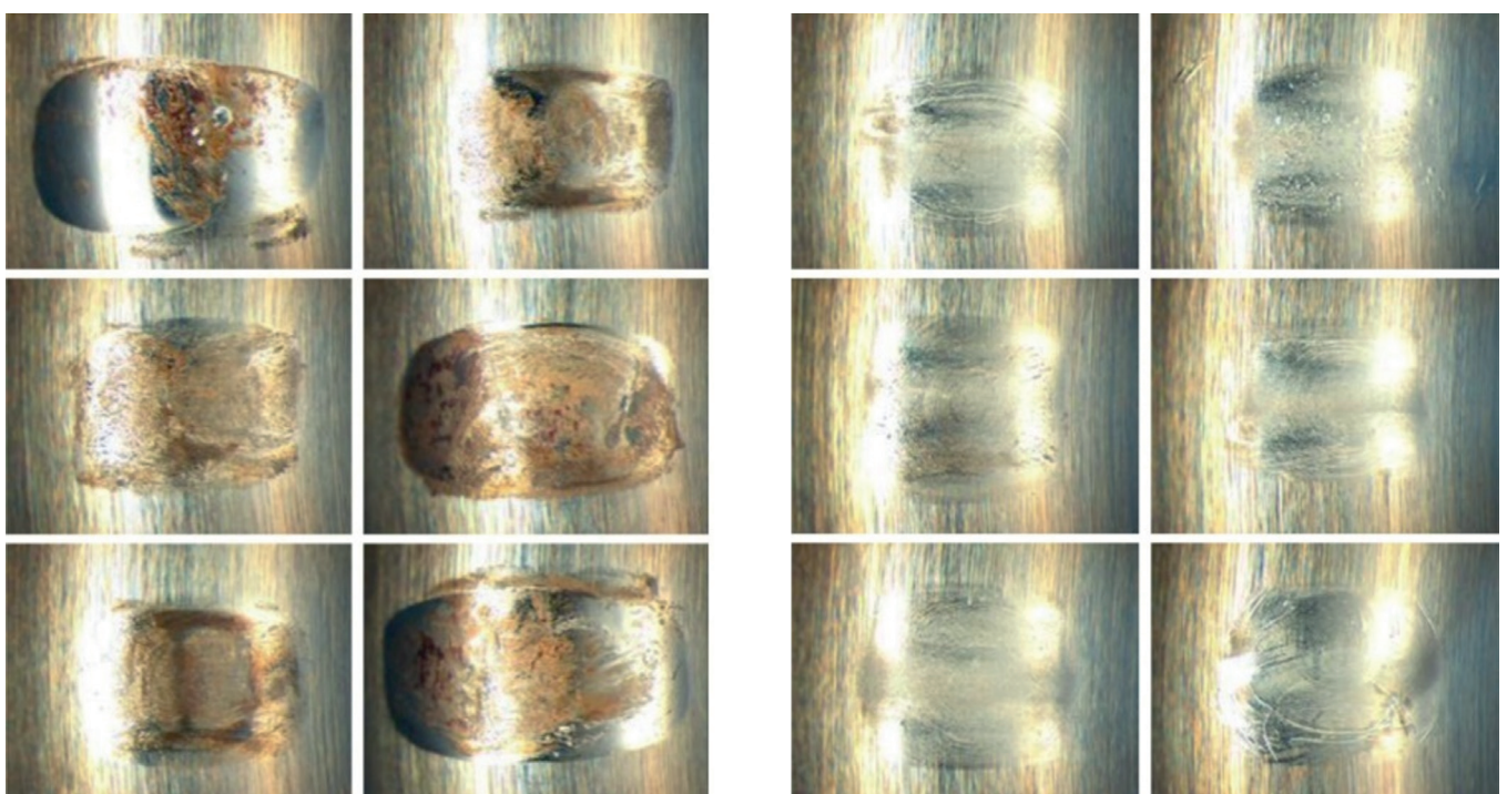
Figure 4: Standstill damages generated through a so called false-brinelling-test without (left) and with (right) the addition of REWITEC.
