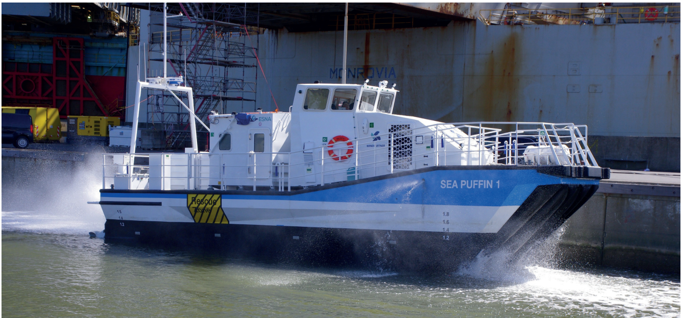
The Sea Puffin 1 demonstrating full air cushion lift. Without the air cushion the draught is just where the black antifouling meets the white side paint.
