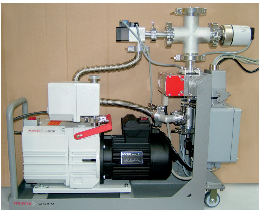
Fig. 1 Customized pumping cart for solar receiver degassing
